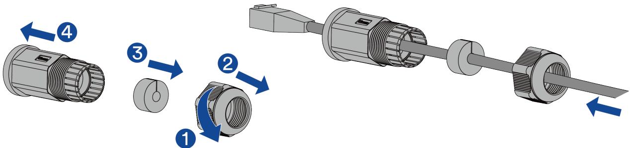
**Step 4:** Connect the “Link Port In” of the BCU to the BMS port of the inverter using a shielded CAT 5 (or higher) ethernet cable. Tighten the cable gland and the insulator.
