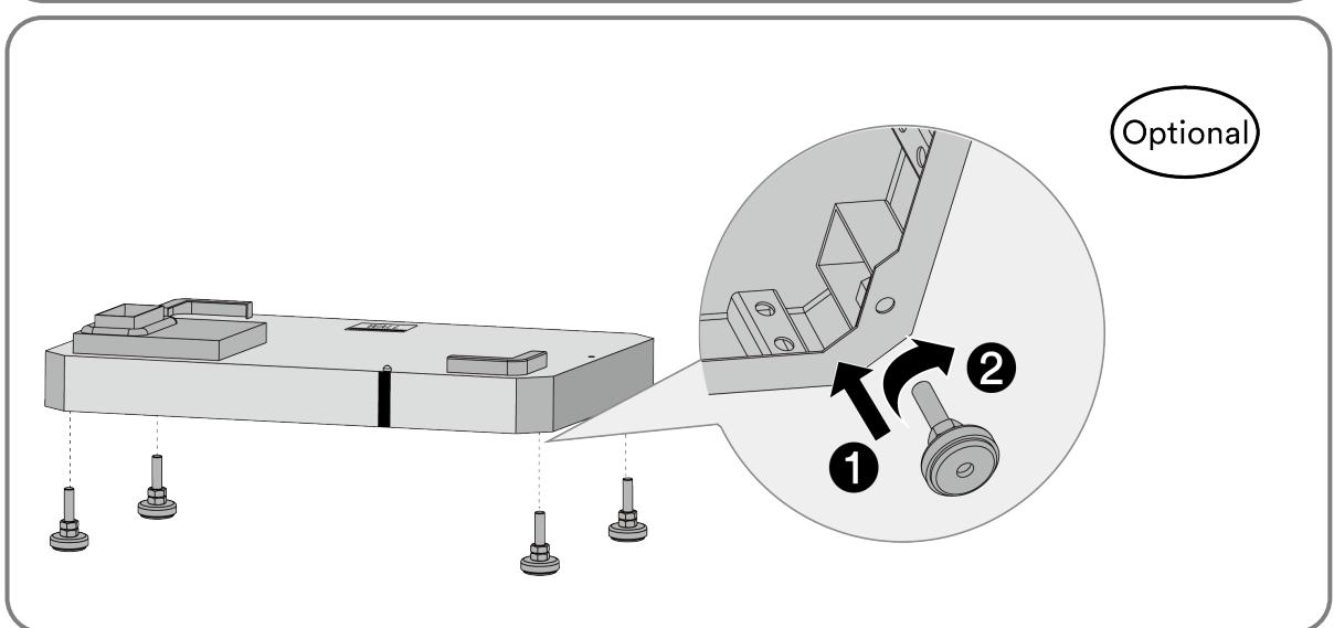
**Step 2:** Place the base along the wall, and ensure a distance of 40~50 mm between the wall and the base. Pay attention to the direction of the base. The power-mating connectors on the base should be on the outside.
