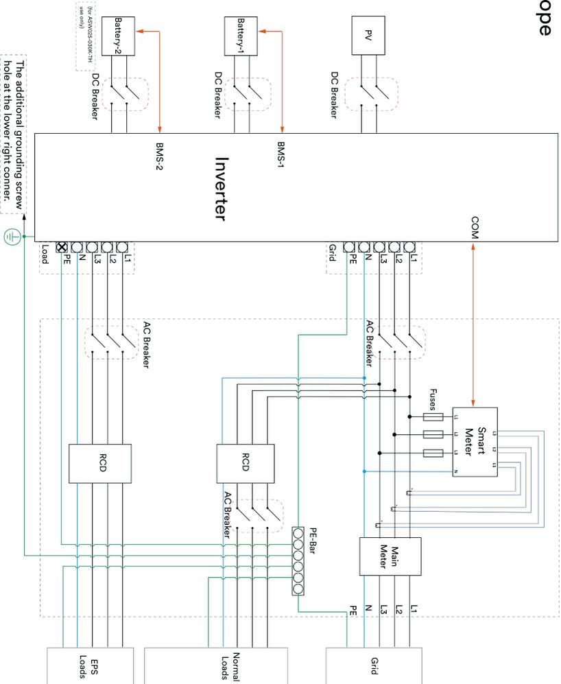
The wiring of a basic application as an example for grid connected systems without special requirements is shown below:
