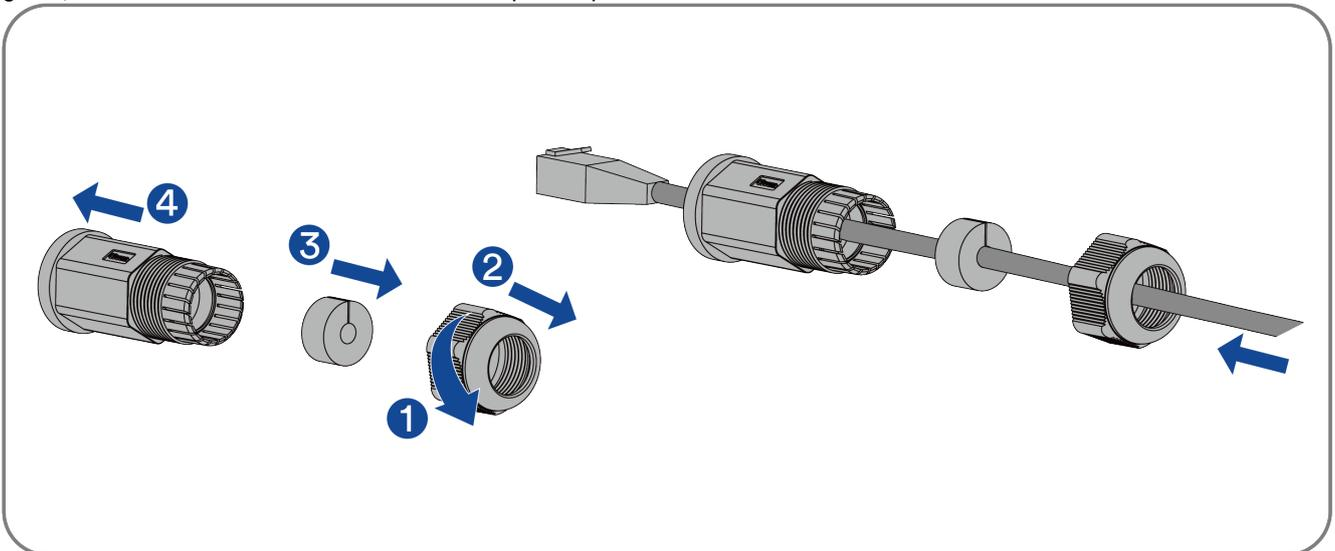
**Step 4:** Connect the “Link Port In” of the BCU to the BMS port of the inverter using a shielded CAT 5 (or higher) ethernet cable. Tighten the cable gland and secure the insulator.
