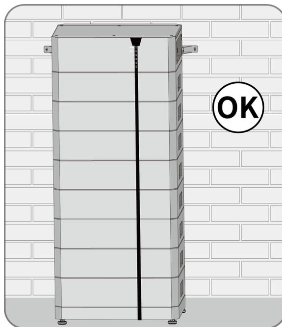
**Step 10:** Secure the hanger using the supplied screws (M8x40).
