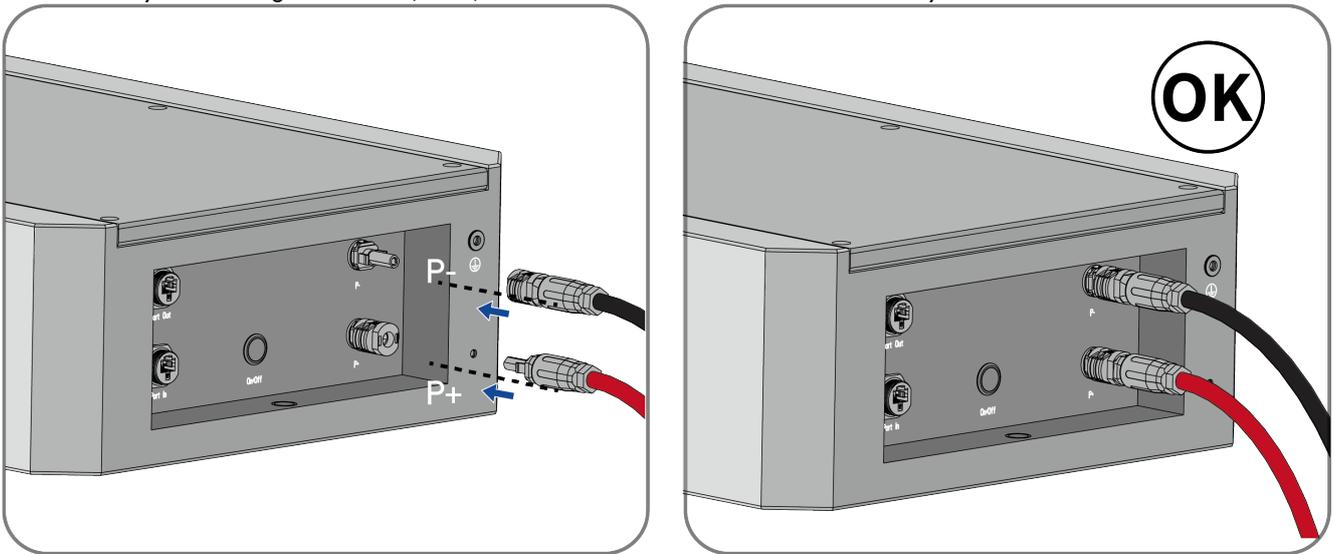
**Step 2:** Attach the connector (supplied in the inverter package) to the opposite ends of the power cables, and connect them to the inverter's battery input connectors.
