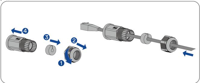
**Step 4:** Connect the "Link Port In" of the BCU to the BMS port of the inverter using a shielded CAT 5 (or higher) ethernet cable. Tighten the cable gland and the insulator.
