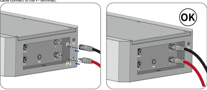
**Step 2:** Add the connector from the inverter package to the opposite ends of the power cables and connect them to the inverter battery input connectors.
