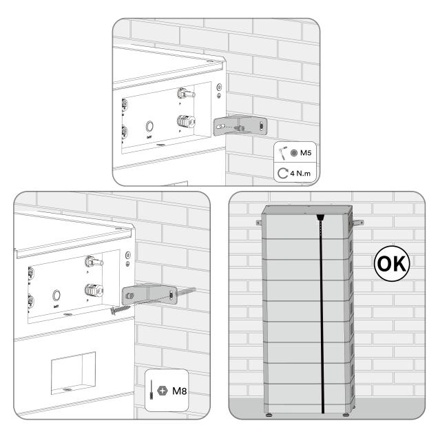
**Step 10:** Secure the hanger using screws(M8×40). **Complete the installation.**
