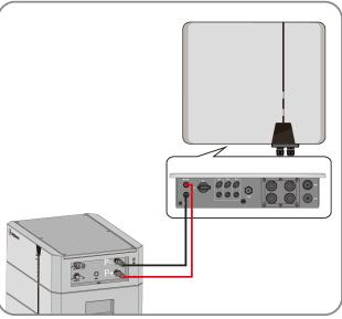
**Step 3:** Split the connectors. Lead the network cable through cable gland, and insert into the insulator until it snaps into place.
