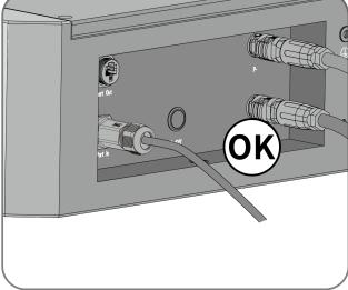
Step 5: Connect the terminating resistor to the "Link Port Out" of the BCU.
