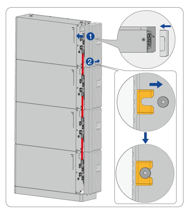
**Step 5:** Secure the decorative covers using the supplied M5×16 screws. The recommended tightening torque is 4 N·m.
