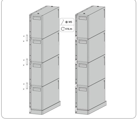
**Step 6:** Hold the L-bracket where it intends to be mounted on the wall and mark the position of the holes. Please pay attention that there may be power cables or other supply lines (e.g., gas or water) routed in the wall. Ensure that no cables or other supply lines are laid in the wall, which could be damaged when drilling holes. Repeat on the other side of the battery.
