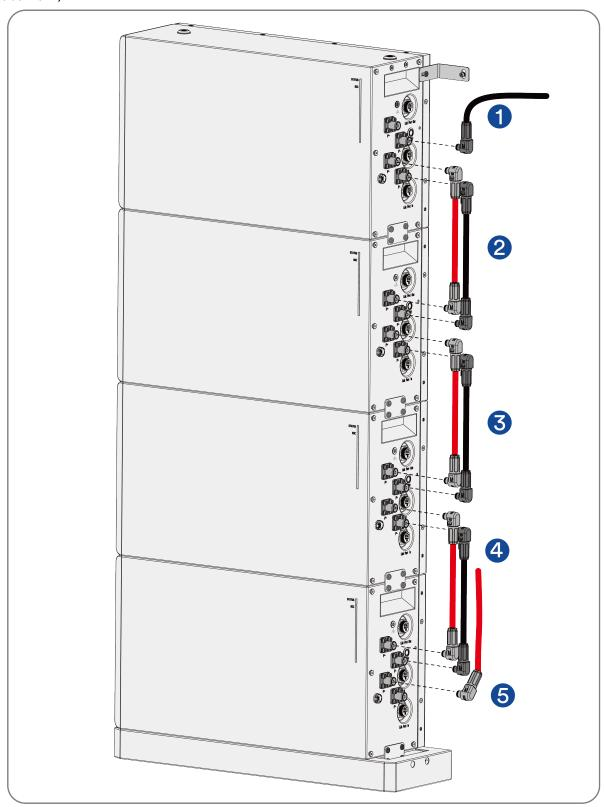
**Step 2:** Connect the "Link Port Out" of the top battery to the BMS port of the hybrid with the supplied output communication cable(2m). Connect the "Link Port In" and "Link Port Out" between the stackable parallel battery modules using the supplied parallel communication cable. Connect the bottom battery "Link Port In" with the supplied terminal resistor.
