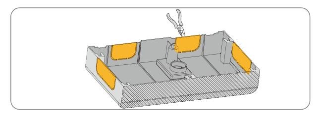
**Step 4:** Align the decorative covers with the cable area of the battery modules, ensuring they fully cover all visible cables. Push the covers towards the battery modules until they fit tightly. Then, slide the covers backward so the internal bayonets on the decorative covers lock securely into the circular slots on the battery modules. Make sure the covers are firmly attached and properly aligned for a neat and secure finish.
