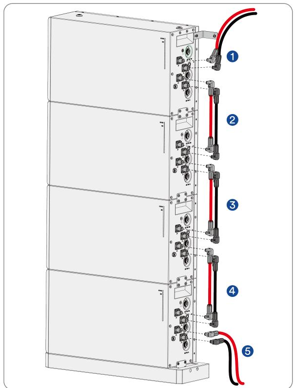
Step 2: Connect the "Link Port Out" of the uppermost battery module to the inverter's battery port using the supplied communication cable. Connect the "Link Port Out" and "Link Port In" of the mid-layer modules with the supplied parallel communication cable. Use the provided terminal resistor to close the "Link Port In" on the lowest module.
