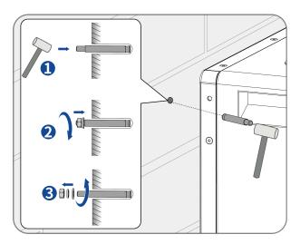
**Step 9:** Secure the L-brackets to both sides of the battery using the supplied screws (M5×10). Tighten with a 4mm ratchet wrench (torque: 4 N·m).
