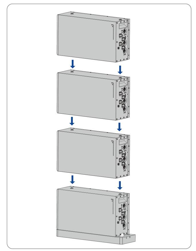
**Step 5:** Repeat the operations for the remaining battery modules.
