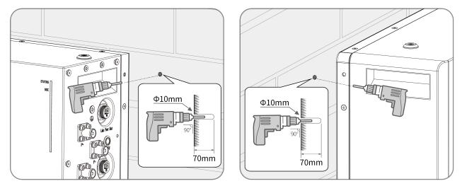
**Step 8:** Clean the dust in the hole, plug the expansion bolt into the hole, fix them with a rubber hammer, and tighten the nuts with a wrench, fix the bolt tail, and remove the nut, spring washer and flat washer and reserve them for the next step. Repeat on the other side of the battery.
