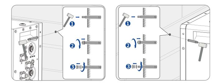
**Step 9:** Fix two L-brackets on both sides of the battery with the supplied screws(M5×10), using a Ratchet wrench (4mm) to tighten it (torque: 4 N.m).
