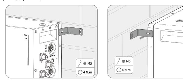
**Step 10:** Fix the L-brackets with the expansion bolts.
