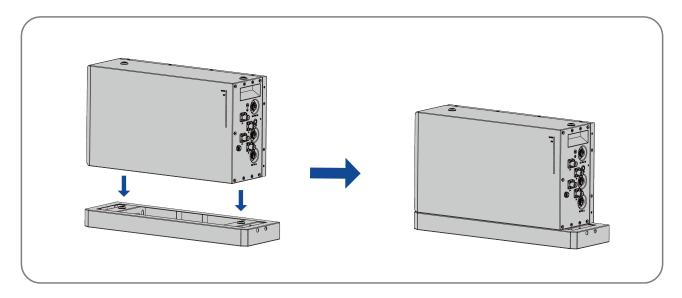
**Step 3:** Install the right anti-tipping bracket, using the module locking plate (right) to align the screw holes from above. Use four screws (M5x10) to secure the module lock plate (right), tightening torque :4 N.m.
