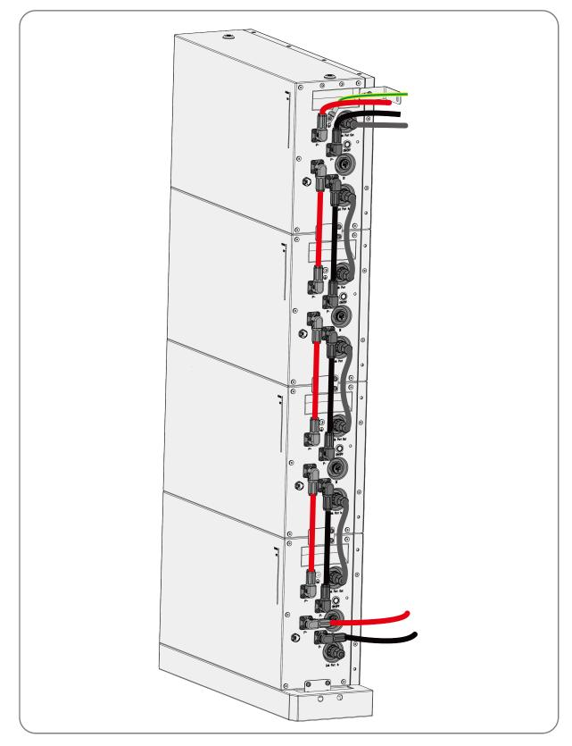
**Step 3:** Cut the cable hole according to the wiring mode.
