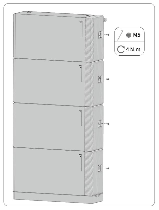
**Step 5:** Secure the decorative covers by the supplied screws(M5×16). Tightening torque: 4 N.m.
