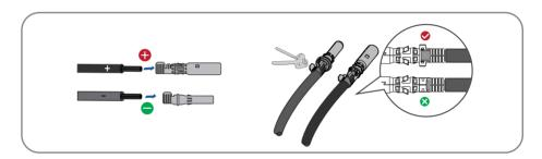
**Step 3**: Insert the cable through cable gland, and insert into the housing until it snaps into place. Gently pull the cable backward to ensure firm connection. Tighten the cable gland and onto the housing (Torque 2.5-3Nm).
