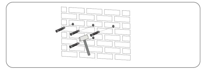
Step 3: Align the mounting-bracket with the hole position and use the tapping nail to fix the hanging plate.
