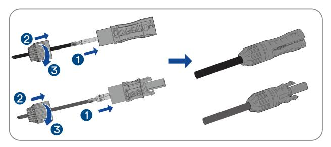
**Step 4:** Ensure that the cable is correctly positioned.
