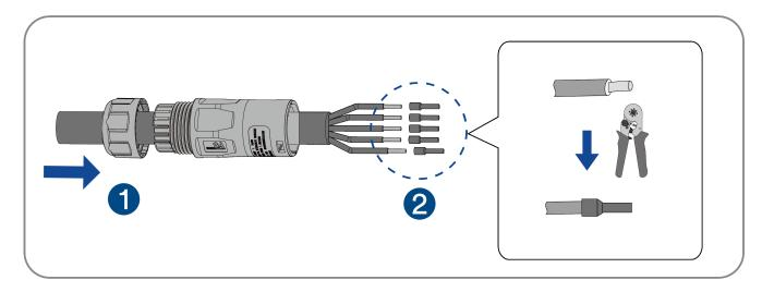
Crimping tool selection and crimping requirements are shown in the following figure:
