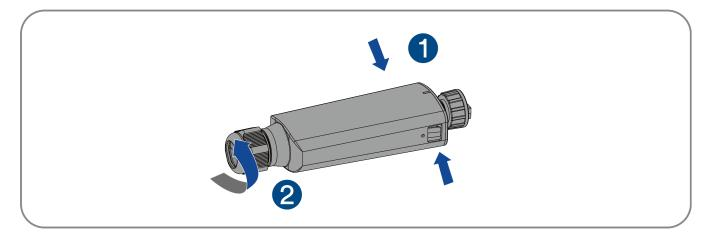
Step 2: Lock the communication cable to the wiring terminal according to the sequence shown in the following figure.
