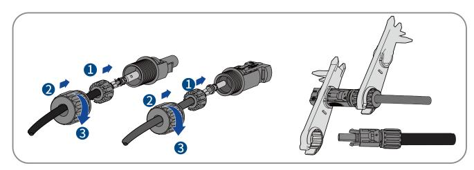
**Step 4:** Ensure that the cable is correctly positioned.
