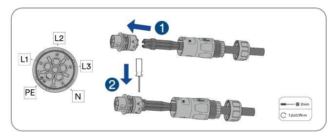
**Step 5:** Insert the main body into the rubber core and hear the "click" sound.
