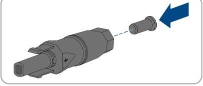
• Insert the DC connectors with sealing plugs into the corresponding DC inputs on the inverter.
