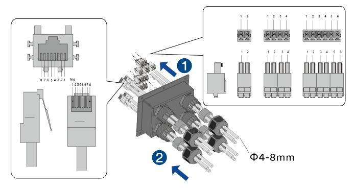
Step 3: Connect the communication cable crimped to the corresponding communication port.
