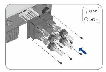
**Step 5:** Tighten the cable gland nuts.
