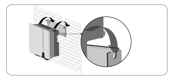
**Step 5:** Fix the inverter with screws.
