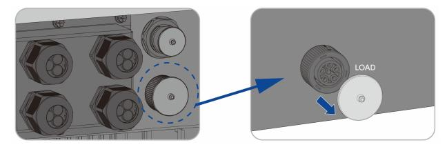
Step 2: The installation arrow indicates insertion the female connector, and hear the "click" sound.
