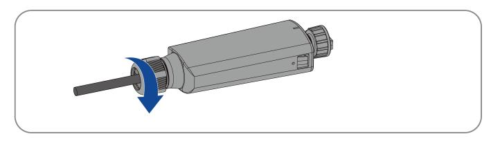
**Step 4:** Remove the dust and waterproof cover of the Ai-Dongle on the inverter and retain it.
