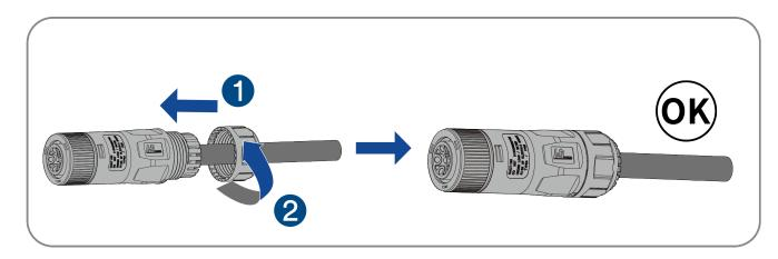
The following figure shows the sequence of the AC connector cable harness.
