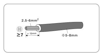
**Step 2:** Assemble the cable ends with the crimping pliers.
