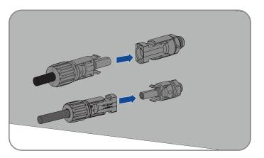
• For unused DC connectors, push down the clamping bracket and push the swivel nut up to the thread. Insert the DC connectors with sealing plugs into the corresponding DC inputs on the inverter.
