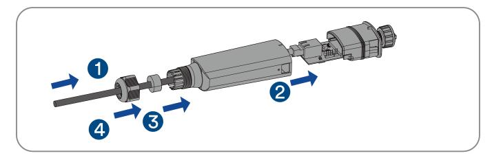
**Step 3:** Insert the wiring terminal into the sealing head, adjust the communication cable, insert the sealing ring, and lock nut.
