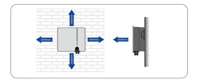
• In case of multiple inverters, reserve specific clearance between the inverters.
