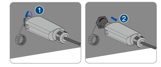
Step 11: Hold down the buckle on the side of the Ai-Dongle and pull out the Ai-Dongle terminal.
