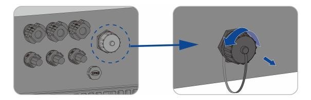
**Step 5:** Attach the Ai-Dongle to the connection port in place and tighten it into the port by hand with the nut in the modular. Make sure the modular is securely connected and the label on the modular can be seen.
