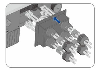
Step 4: Install the communication cover on the inverter.
