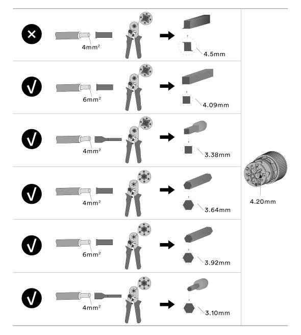
**Step 4:** Set the parts on the cable, insert the terminal holes in sequence. Crimp the wire with an inner hexagon screwdriver and screw the torque 1.2+/-0.1N·m.
