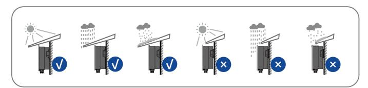
Never install the inverter horizontally, or with a forward / backward tilt or even upside do- wn. The horizontal installation can result in damage to the inverter.
