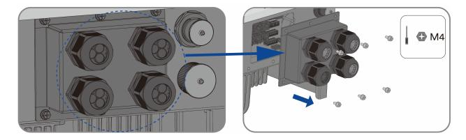
**Step 2:** Route the communication cable through the communication cover and crimp the wiring terminal.
