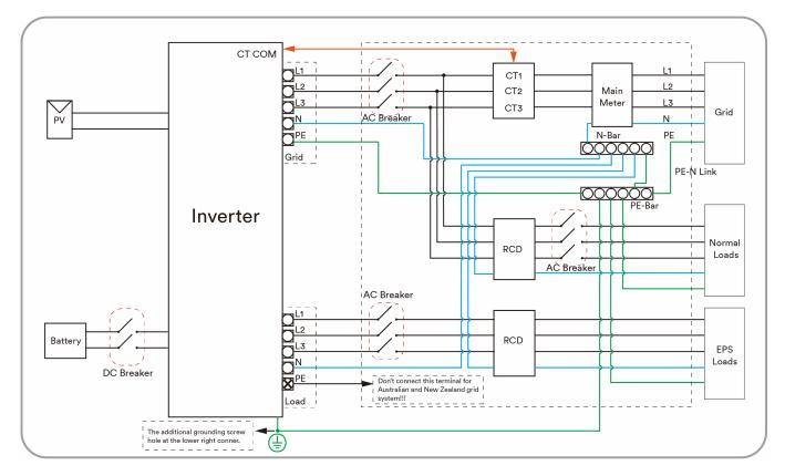
For other countries, the following diagram is an example for grid systems without special requirement on wiring connection.
