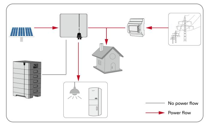
Case 3: The battery discharge when the utility grid loss.
