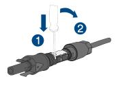
Remove the cable and go back to step 2.
