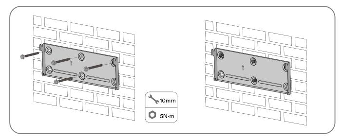
**Step 4:** Hang the inverter to the mounting-bracket and ensure that the mounting ears perfectly engage with the mounting-bracket.
