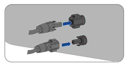
• For unused DC connectors, push down the clamping bracket and push the swivel nut up to the thread. Insert the DC connectors with sealing plugs into the corresponding DC inputs on the inverter.
