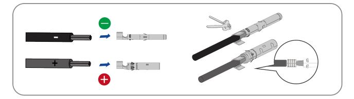
**Step 3:** Lead the cable through cable gland, and insert into the insulator until it snaps into place. Gently pull the cable backward to ensure firm connection. Tighten the cable gland and the insulator (Torque 4Nm).
