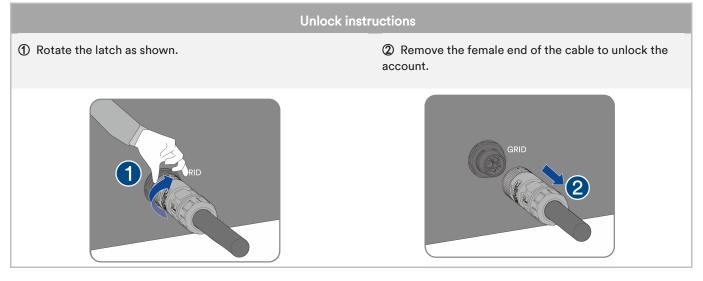
Step 8: Loosen and remove the EPS Load connector.
