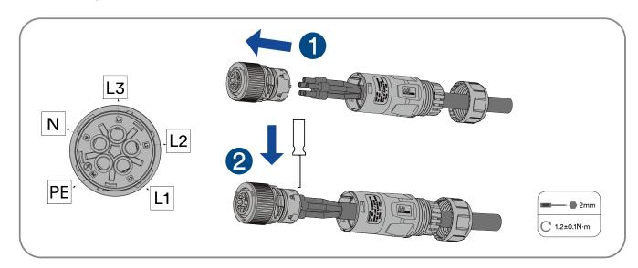
**Step 5:** Insert the main body into the rubber core and hear the "click" sound.
