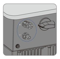
Step 2: Connect the assembled DC connectors to the inverter.
