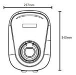
A solid, flat support surface, e.g., concrete or masonry, must be available for mounting.
