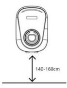
The installation location must be freely accessible.
