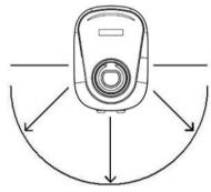
The mounting location must be selected so that the EV Charger and the vehicle can be connected with the charging cable without exerting undue stress on the charging cable.
