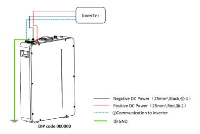
Fig. 4.1.1 Single-Set System Cable Connection Diagram (5kWh,Output Power 2.5kW)
