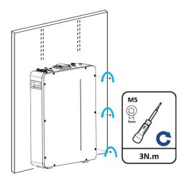
Fig.5.2.1 Take down battery front panel
