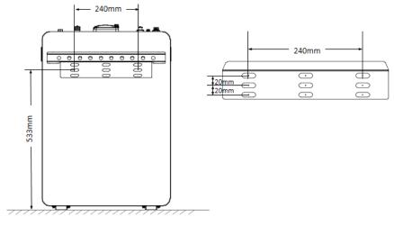
Fig. 4.2.1 Installation hole size
