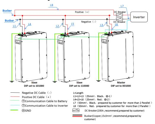
Fig. 5.1.1 Multi-Sets Connection (Example: 3 Parallel, 15kWh, Output Power 7.5kW) (Battery  $\Delta V$  should be less than 3V at first Parallel installation)
