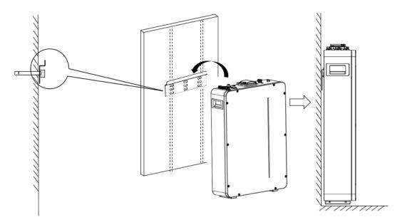
Fig. 4.2.3 Installation battery
