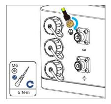
Fig. 4.3.3 Ground cable connection
