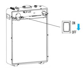
Fig5.2.2 Turn off the internal battery
