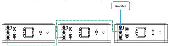
Fig. 5.3.1 Communication cable connection
