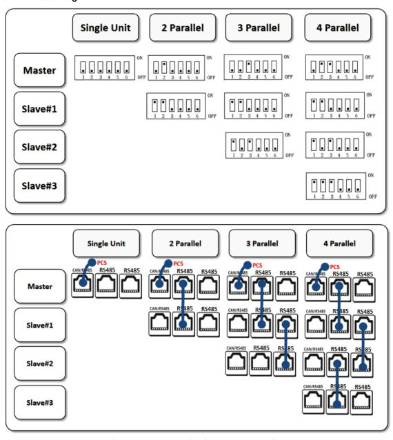
Fig. 5.4.2- Communication port connecting (If more than 4 LB51100A in parallel, please contact the engineer of supplier.)
