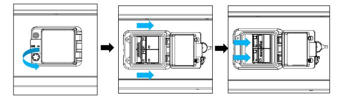
Fig. 4.4.1 Procedure for opening the circuit breaker protective cover
