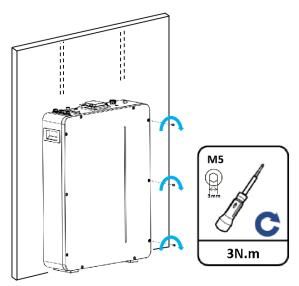
Fig.5.6.1 Install the front panel
