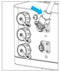
Fig. 4.3.5 Power cable connection
