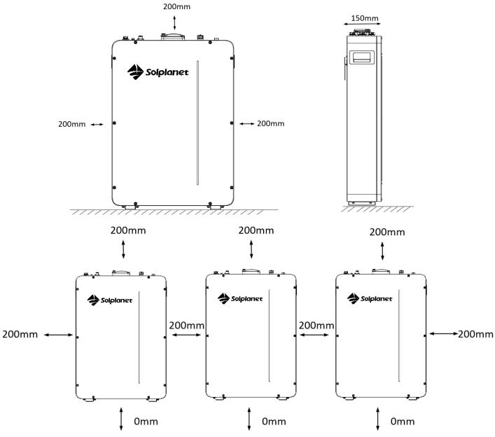
Fig. 3.4.1 Space Requirements Schematics
