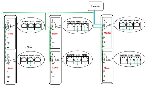
Fig. 5.3.1 Communication cable connection-3 Parallel(30kWh)
