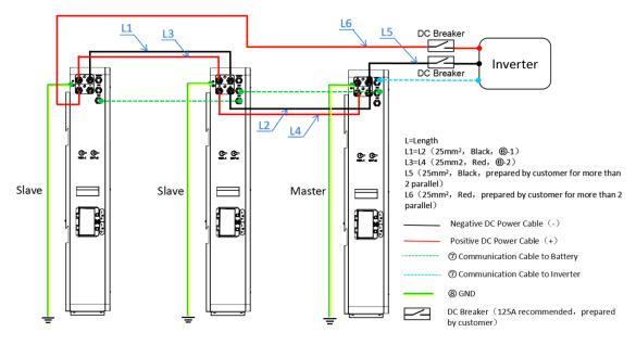
Fig.5.1.1 Multi-Sets Connection(Example: 3 Parallel, 30kWh, Output Power 5kW) (Battery  $\Delta V$  should be less than 3V at first Parallel installation)
