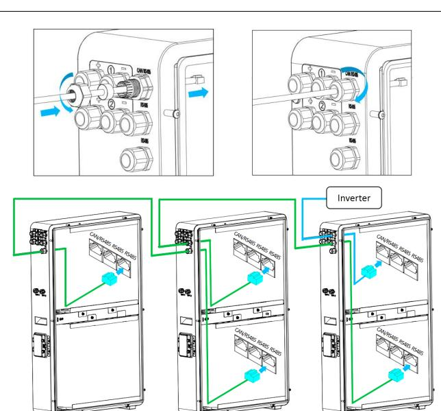
Fig.5.3.2 Communication cable connection
