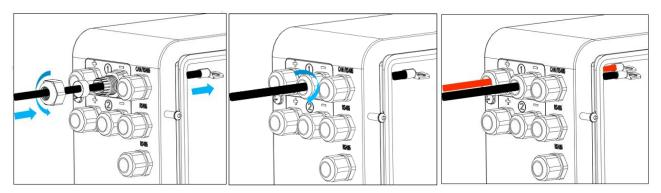
Fig.5.3.3 Power cable connection
