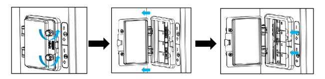
Fig. 4.4.1 Procedure for opening the circuit breaker protective cover
