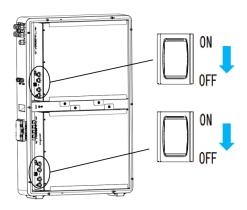
Fig5.2.2 Turn off the internal battery
