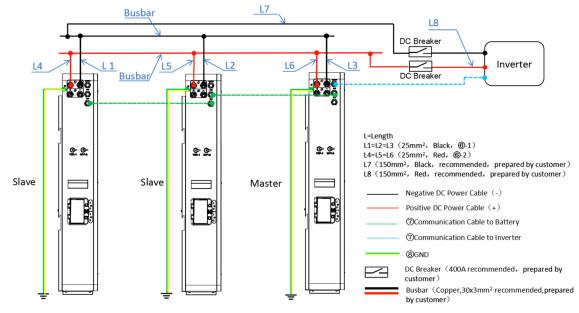
Fig.5.1.2 Multi-Sets Connection(Example: 3 Parallel,30kWh,Output Power 15kW) (Battery ΔV should be less than 3V at first Parallel installation )
