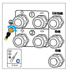
Fig. 4.3.1 Ground cable connection
