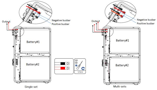
Fig. 5.3.4 DC Output Power Cable Wiring diagram
