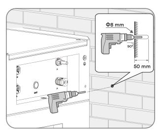
**Step 8:** Insert a screw anchor into the hole. Repeat on the other side of the BCU.
