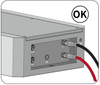
**Step 2:** Add the connector from the inverter package to the opposite ends of the power cables and connect them to the inverter battery input connectors.
