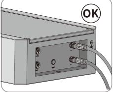
**Step 3:** Split the connectors. Lead the network cable through cable gland, and insert into the insulator until it snaps into place.
