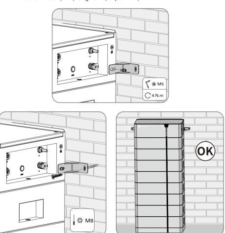
Step 10: Secure the hanger using screws(M8×40).
