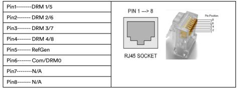
If DRMs support is required, the inverter should be used in conjunction with AiMonitor. the Demand Response Enabling Device (DRED) can be conneted to the DRED port on AiMonitor via RS485 cable. You can vist the website <u>www.solplanet.net</u> for more information and download the user manual for the AiMonitor.
