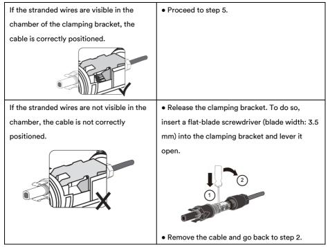
5.6.3 Disassembling the DC connectors
