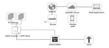
The smart meter should support the MODBUS protocol with a baud rate of 9600 and address set 1. Smart meter as above SDM230-Modbus connecting method and seting baud rate method for modbus please refer to it's user manual.
