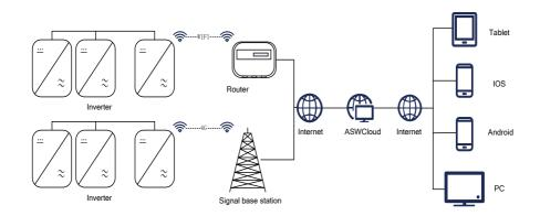
Method 1 only one inverter with the 4G/WiFi Stick, the other inverter be connected through the
