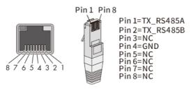
4. Unscrew the communication port cover cap in the following arrow sequence and insert the network cable into the RS485 communication client attached.
