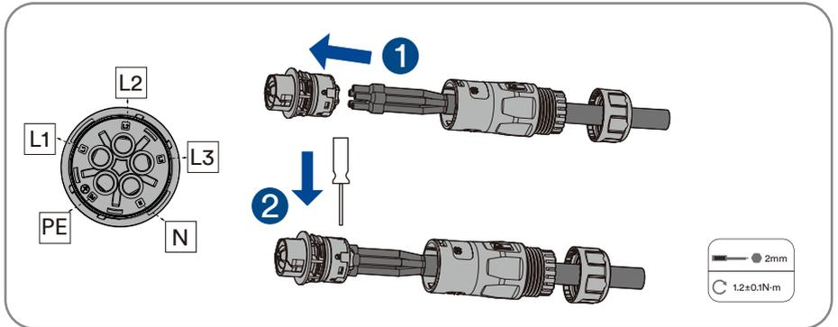
**Step 5:** Insert the main body into the rubber core and hear the “click” sound.
