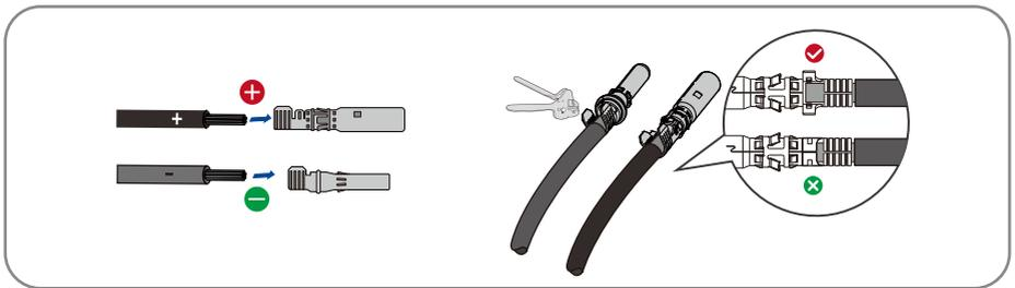
**Step 3:** Lead the cable through cable gland, and insert into the insulator until it snaps into place. Gently pull the cable backward to ensure firm connection. Tighten the cable gland and the insulator (Torque 2.5-3Nm).
