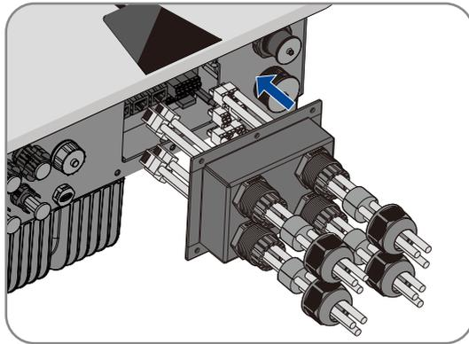
**Step 4:** Install the communication cover on the inverter.
