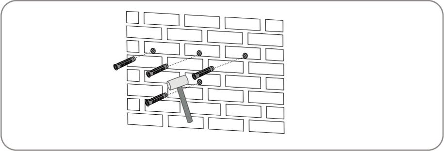
**Step 3:** Align the mounting-bracket with the hole position and use the tapping nail to fix the hanging plate.
