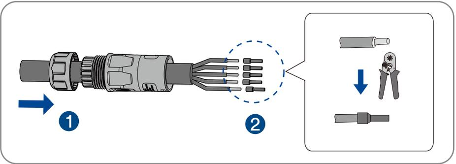
**Step 4:** Set the parts on the cable, insert the terminal holes in sequence. Crimp the wire with an inner hexagon screwdriver and screw the torque  $1.2 \pm 0.1 \text{ N}\cdot\text{m}$ .
