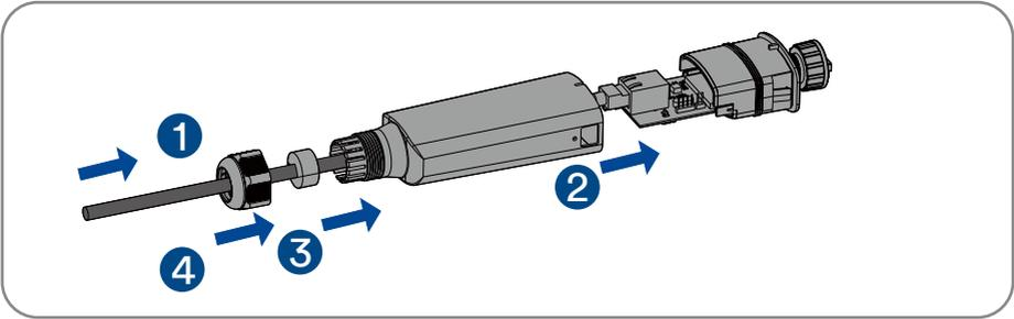
**Step 3:** Insert the wiring terminal into the sealing head, adjust the communication cable, insert the sealing ring, and lock nut.
