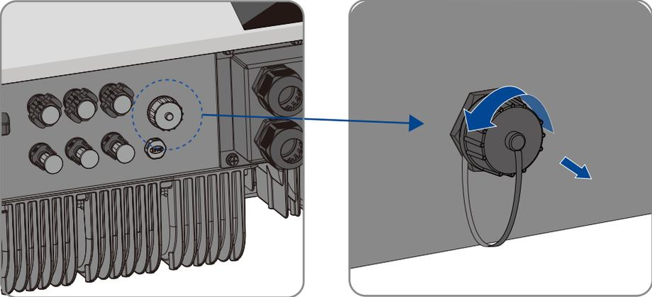
**Step 5:** Attach the Ai-Dongle to the connection port in place and tighten it into the port by hand with the nut in the modular. Make sure the modular is securely connected and the label on the modular can be seen.
