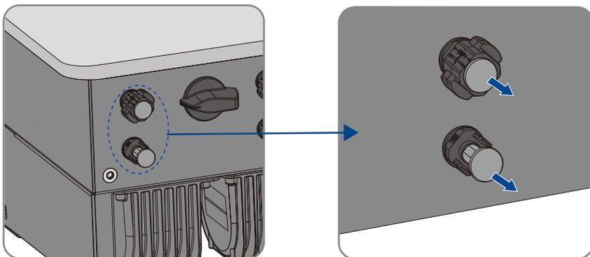
**Step 3:** Connect the assembled DC connectors to the inverter.
