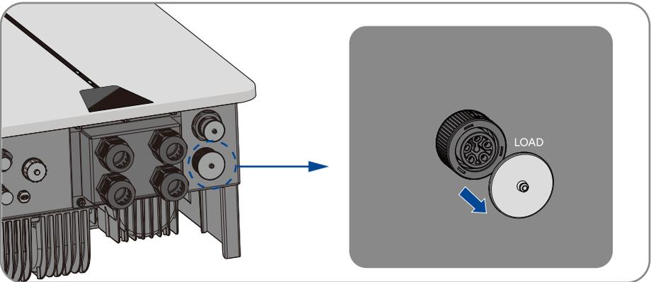
**Step 2:** The installation arrow indicates insertion the female connector, and hear the “click” sound.
