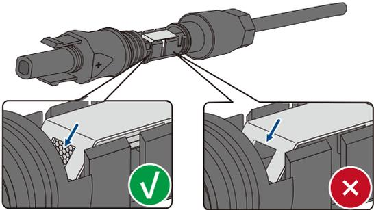
Release the clamping bracket. To do so, insert a screwdriver (blade width: 3.5mm) into the clamping bracket and pry the clamping bracket open.
