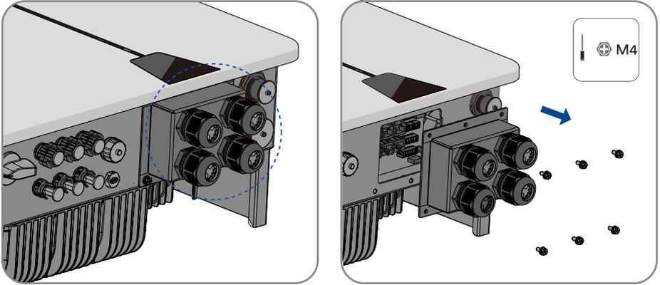
**Step 2:** Route the communication cable through the communication cover and crimp the wiring terminal.
