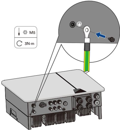
**Step 3:** Apply paint to the grounding terminal to ensure corrosion resistance.
