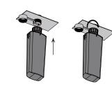
To remove the Stick from the inverter, turn the floating screw counterclockwise as shown in the figure below. After removing the Stick, tighten the anti-dust cap clockwise to ensure inverter protection.
