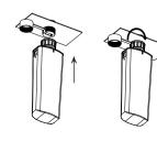
To remove the Stick from the inverter, turn the floating screw counterclockwise as shown in the figure below. After removing the Stick, tighten the anti-dust cap clockwise to ensure inverter protection.
