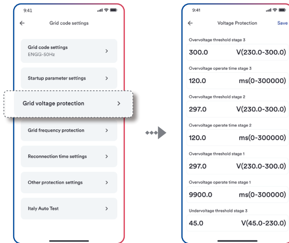
Figure 18. Grid voltage protection settings
