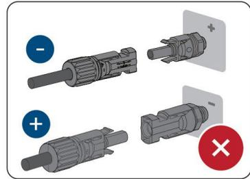
**Step 7:** Ensure that all DC connectors and the DC connectors with sealing plugs are securely in place.
