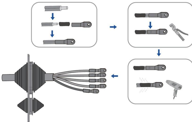
**Step 9:** Secure the wires to corresponding terminals.
