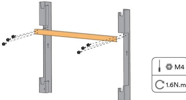
**Step 2:** Align the wall mounting bracket horizontally on the wall with the arrow upwards. Mark the position of the drill holes. Set the wall mounting bracket aside and drill the marked holes with the diameter of 12mm. The depth of the holes should be about 65 mm. Keep the hammer drill bit perpendicular to the wall to avoid drilling inclined.
