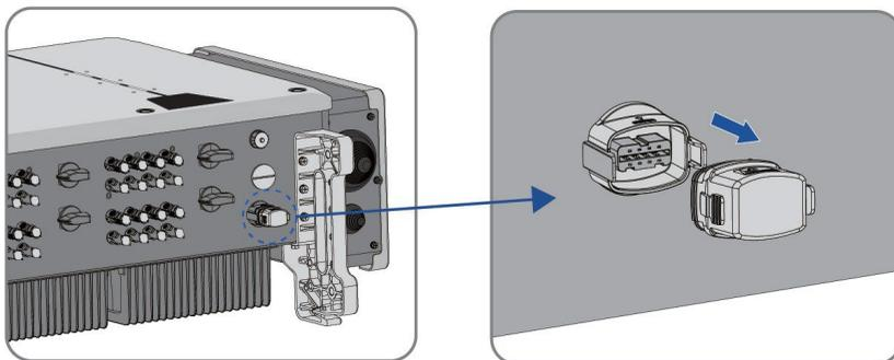
**Step 3:** Rotate the nut, take out the sealing ring, take out the plug, hold the locking structure, and take out the wiring terminal.
