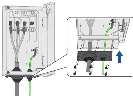
**Step 11:** Close the wiring compartment and tighten the two screws on the wiring compartment with a torx screwdriver.
