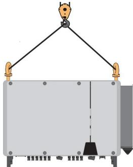
**Step 4:** Remove the lifting ring.
