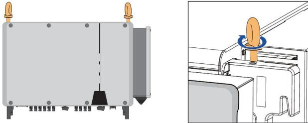
**Step 2:** Lead the sling through the two lifting rings and fasten the tie-down strap.
