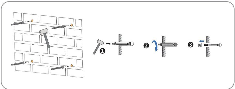
**Step 4:** Fix the mounting-bracket with the expansion bolts.
