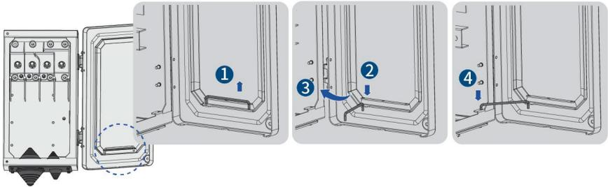
**Step 4:** Use a screwdriver to remove the waterproof ring at the bottom of the wiring compartment and store the removed screws properly.
