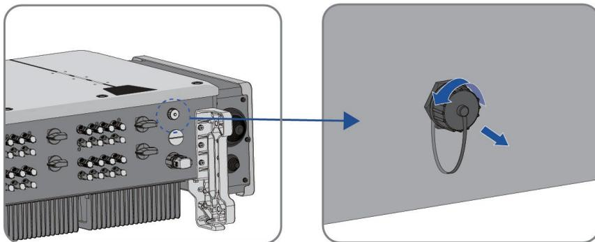
**Step 3:** Attach the WiFi modular to the connection port in place and tighten it into the port by hand with the nut in the modular. Make sure the modular is securely connected and the label on the modular can be seen.
