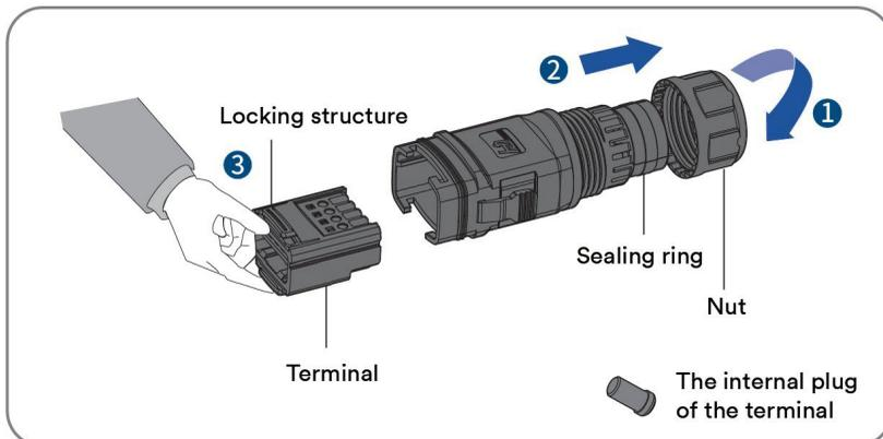
**Step 4** : Lock the shielded twisted-pair communication cable to the wiring terminal according to the sequence shown in the following figure, insert the wiring terminal into the sealing head, adjust the communication cable, insert the sealing ring, and lock the nut.
