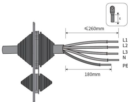
**Step 8:** Make the cable and crimp OT/DT terminal.
