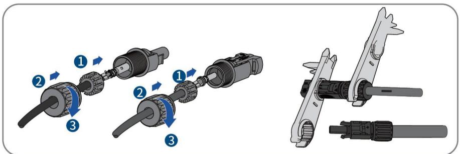
**Step 4:** Ensure that the cable is correctly positioned.
