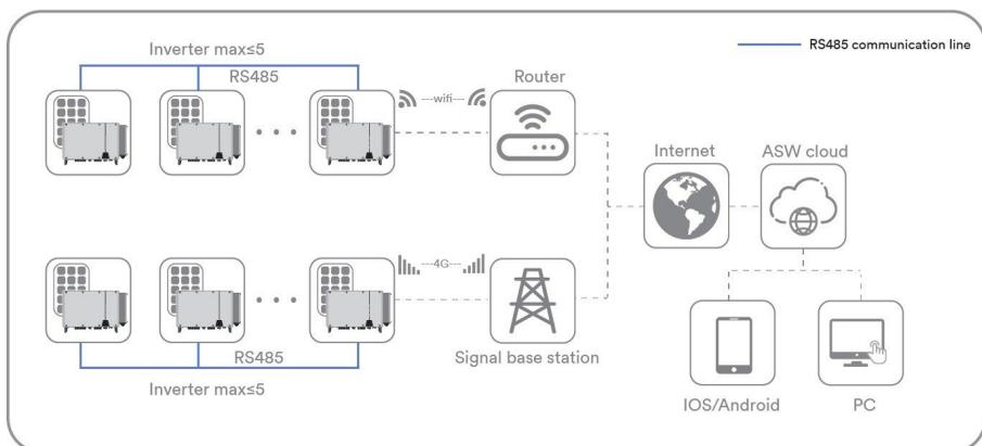
The communication overview with Ai-Logger for large PV plant:
