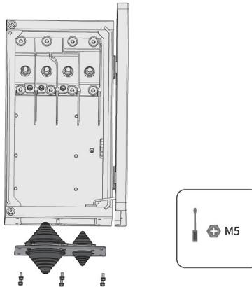
**Step 5:** Cut the appropriate hole in the tower guard coil according to the selected AC wire outer diameter specification.
