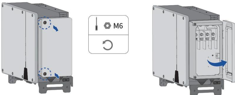
**Step 3:** Keep the wiring compartment opened during wiring through the limit lever attached to the cover.
