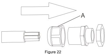
Install the cable gland on the bottom of the enclolsure, fasten the nut (B) and then fasten the nut (A).
