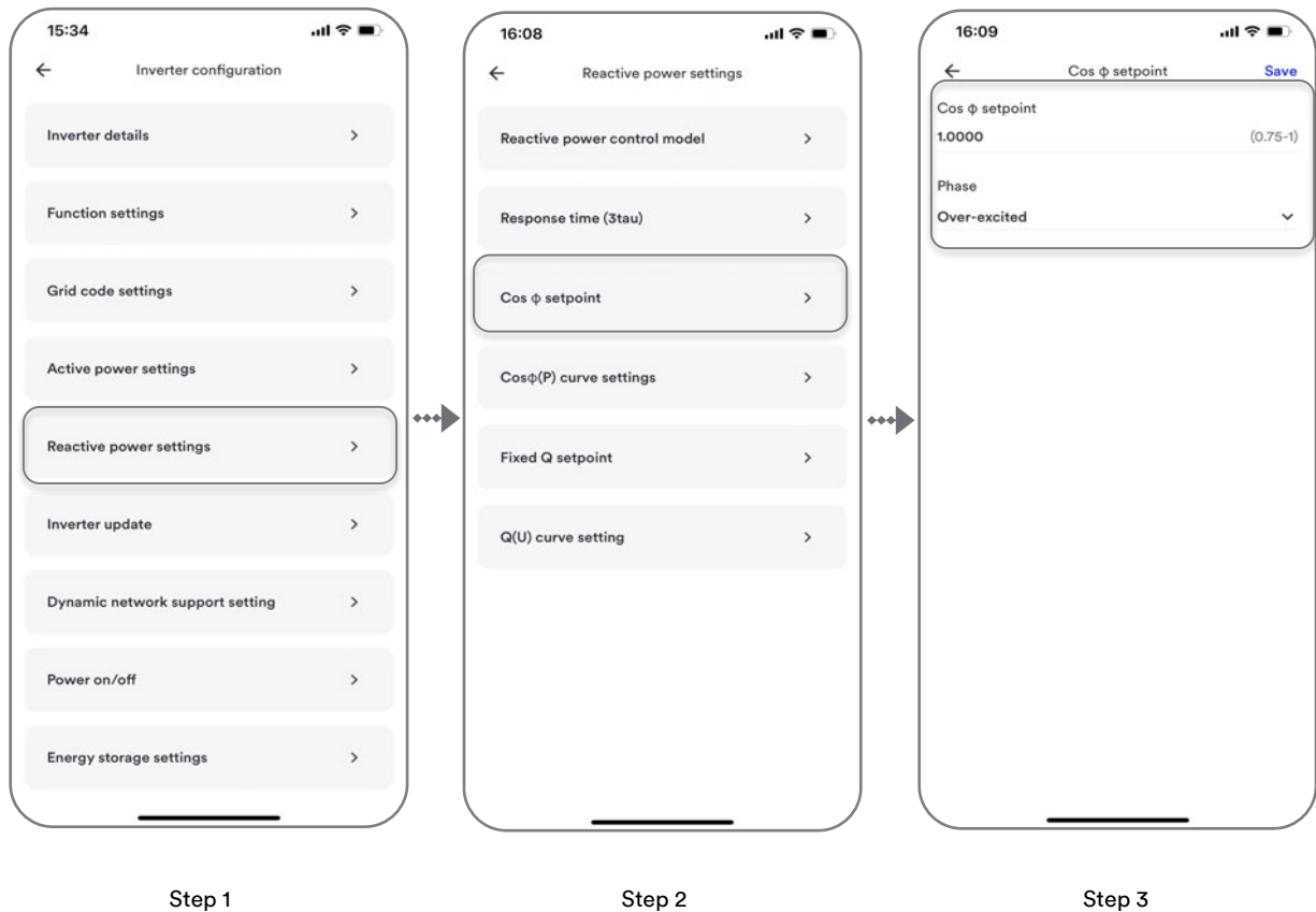
Fig. 58. Define the cos-phi target value
