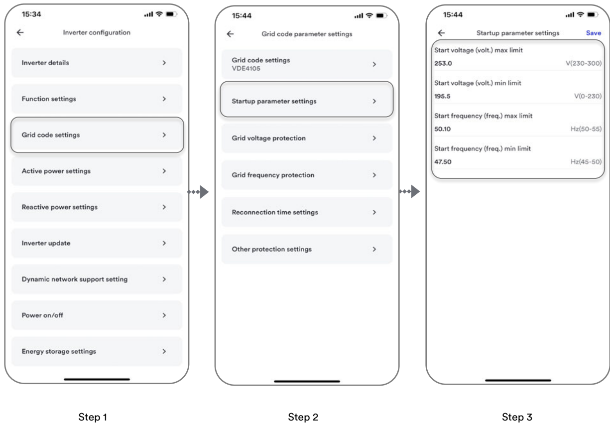
Fig. 19. Set start voltage and start frequency value
