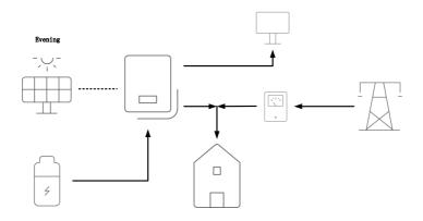
4) In case of the grid failure, switch to off grid, and off grid load can still work normally
