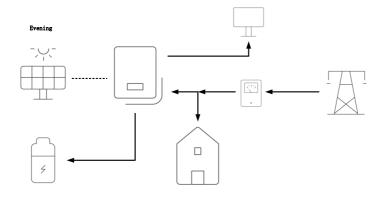
3) When GRID failure and PV energy is unsufficient, the battery supplies power to the load.
