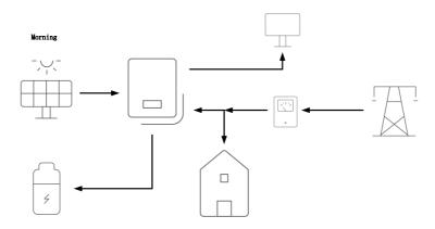
2) Under normal conditions, the battery does not discharge, Even at night.
