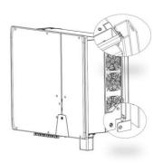
4. Secure the inverter to the mounting bracket on both sides using two M5 screws.
