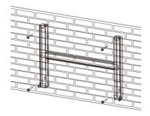
3. Hang the slot on the back of the inverter to the hook on the top of the mounting bracket.
