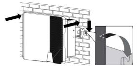
4. Check both sides of the heat sink to ensure that it is securely in place. insert one screw M5x12 each into the lower screw hole on both sides of the inverter anchorage bracket respectively and tighten them.
