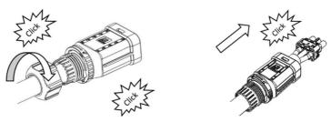
6. Connect the AC connector plug to the inverter's AC output terminal.
