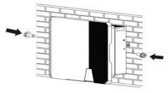
If a second protective conductor is required in installation site, ground the inverter and secure it so that it cannot drop from the housing (see section 5.4.3 "Second protective grounding connection").
