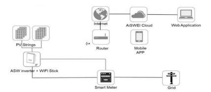
The smart meter should support the MODBUS protocol with a baud rate of 9600 and address set 1. Smart meter as above SDM630-Modbus connecting method and seting baud rate method for modbus please refer to it's user manual.
