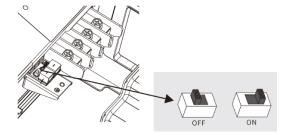
If multiple inverters adopt daisy chain communication configuration, the configuration method of 485 bus matching resistance is suggested as follows:
