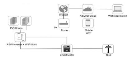
The smart meter should support the MODBUS protocol with a baud rate of 9600 and address set
