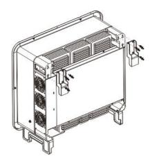
4. Hold the inverter using the handles at the corners, attach the inverter onto the wall bracket tilted slightly downwards.
