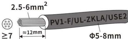
2. Route the stripped cable all the way into the DC connector. Ensure that the stripped cable and the DC connector have the same polarity.
