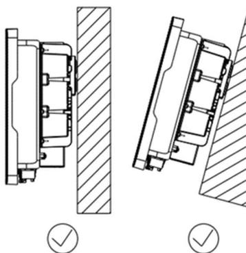
12. Never install the inverter horizontally, or with a forward tilt or with a backward tilt or even with upside down. The horizontal installation can result in damage to the inverter.
