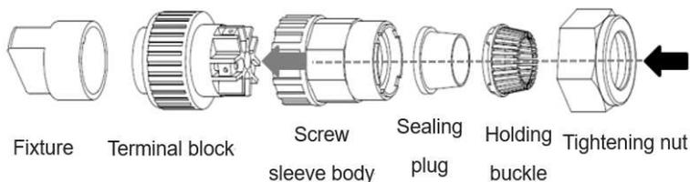
4. Push the holding buckle and the sealing plug into the screw sleeve body, and then assemble the terminal block, the screw sleeve body and the tightening nut together. First clamp the terminal block with a plastic clamp, then screw the screw sleeve body onto the terminal block, and finally tighten the tightening nut.
