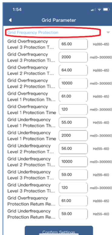
Figure 2-5-18 Grid frequency protection
