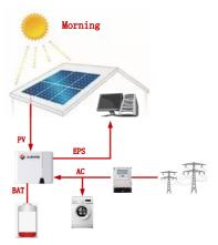
In the afternoon, the photovoltaic energy is sufficient, the load is powered by photovoltaic, the battery is charged, and the excess energy is connected to the Internet.
