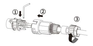
5. Plug the AC connector into the jack for the AC connection and screw tight.
