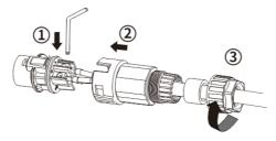
3. Plug the AC connector into the socket for the EPS connection.
