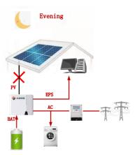
In case of power failure, switch to off grid, and off grid load can still work normally
