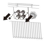
2) Loosen the swivel nut of the cable gland on the communication plate, remove the sealing plug and lead the stripped cable through the swivel nut, sealing sleeve, communication plate and magnetic ring, crimp the crystal as below pin assignment.
