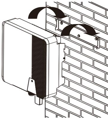
4. Check both sides of the heat sink to ensure that it is securely in place.
