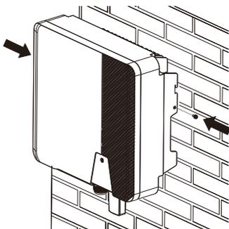
If a second protective conductor is required in installation site, ground the inverter and secure it so that it cannot drop from the housing (see section 5.4.3 “Second protective grounding connection”).
