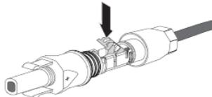
4. Ensure that the cable is correctly positioned:
