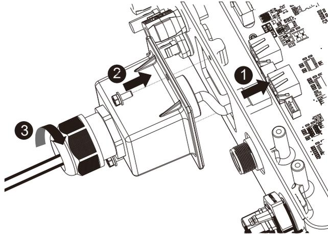
**Disassemble the network cable in reverse order.**
