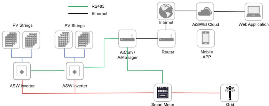
The AiCom/AiManager connects to the inverter via the RJ45 interface, and it connects to the router via Ethernet. User can monitor the inverter through the external AiCom/AiManager with Ethernet module (optional),
