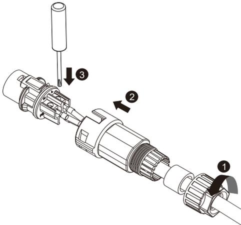
5. Assemble the locking cap, threaded sleeve and swivel nut together. When doing so, hold the bush insert firmly by the locking cap, This ensures that the threaded sleeve can be screwed firmly onto the bush insert. Then screw the threaded sleeve and swivel nut.
