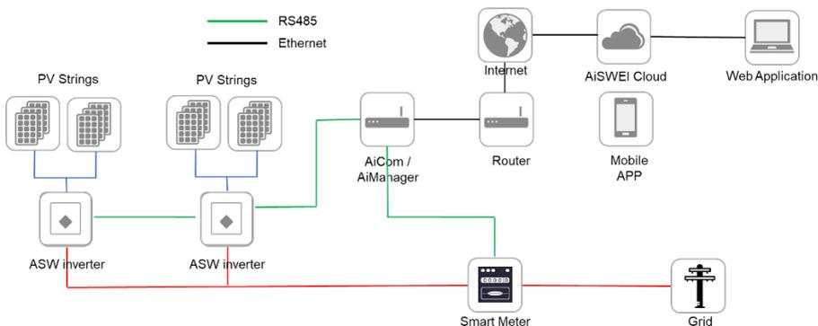
smart meter as above SDM120-Modbus connecting method and setting baud rate method for modbus please refer to its user manual.
