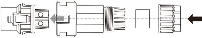
4. Insert the crimped conductors L, N and PE into the corresponding terminals and tighten the screw with a Torx screwdriver(TX 8, torque: 1.4Nm). Ensure that all conductors are securely in place in the screw terminals on the bush insert.
