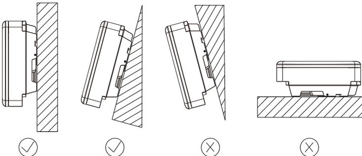
1. Mount the inverter vertically or tilted backward by a maximum of 15°.
