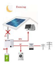
In case of the grid failure, switch to off grid, and off grid load can still work normally
