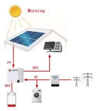
In the afternoon, the photovoltaic energy is sufficient, the load is powered by photovoltaic, the battery is charged, and finally exported to the grid.
