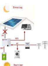
3) When there is a GRID failure, the battery supplies power to the load.
